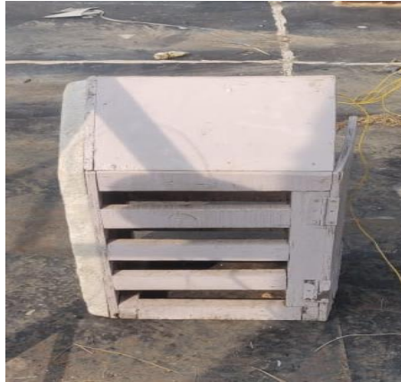
Figure 3.7 Setup for measuring the ambient Temperature
