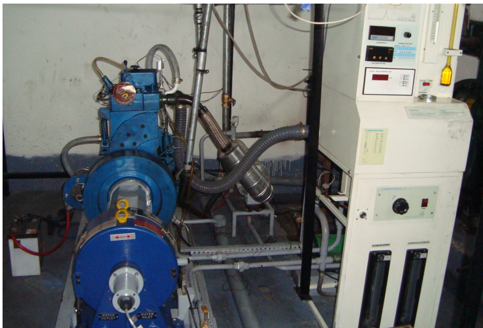
Fig. 2 Variable compression ratio engine test bench
