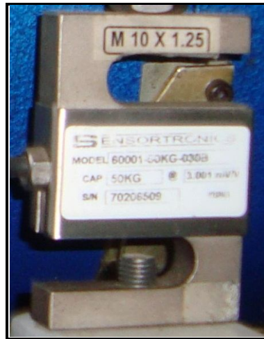
Figure 3.5: Load cell type strain gauge, make sensortronics
