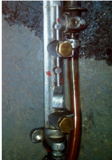
Figure 3.19: Modified Fuel Accumulator.
