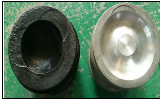
Figure 3.34: Actual and modified piston bowl design.
