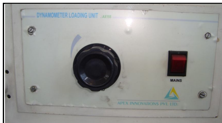
Figure 3.6: Engine loading unit
